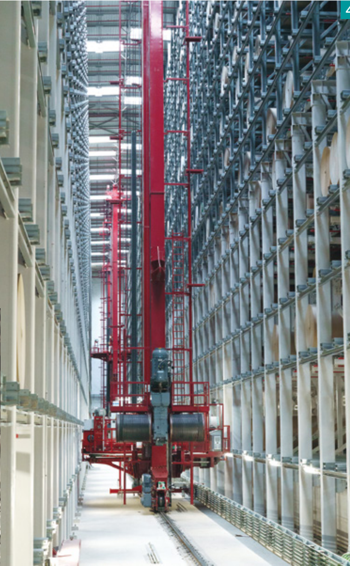
4. Automated high bay warehouse at Saica El Burgo de Ebro mill in Spain.
