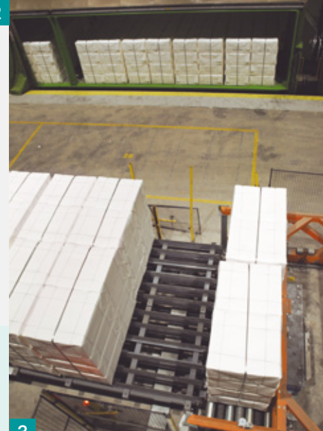
3. Unmanned high-bay pulp warehouse and distribution center with automated train loading.
